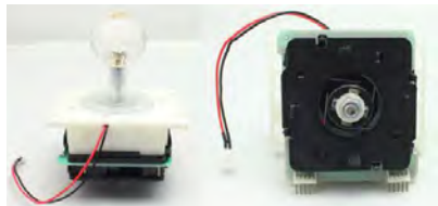
Switch with PCB and LED light
